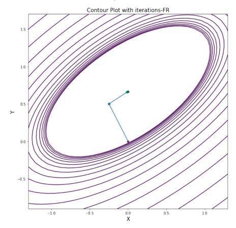
**Observations:** The algorithm almost reaches the optimal point in just two iterations which verifies the result that the algorithm converges in n (here 2) iterations in case of quadratic functions. Now in order to compare the directions obtained by the two methods - DFP and FR, we compute the norm of the difference of the two and have obtained the following result -
