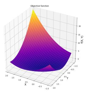
The above plot along with the form of the objective function f(x) makes it very clear that it is convex and moreover it is quadratic in nature. Before implementing the two methods mentioned above we compute the expressions for the gradient and hessian of the objective function.
